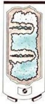
Water heater with hard water scale build-up
